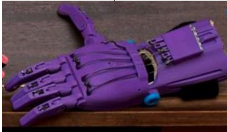
Figura 6. Prótesis de agarre con dedos separados Raptor Reloaded (Enabling the Future, 2015). Tomado de Design and Development of an Upper Limb Prosthesis Vanessa Mariana Alves Carvalho Lopes
